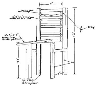
FIGURE 35.—Equipment for reaction test.
